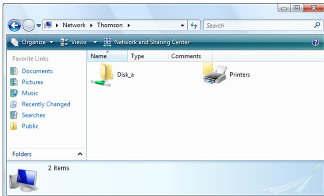
If the storage device has multiple partitions an index number will be added at the end (for example: Disk\_a1 and Disk\_a2).
