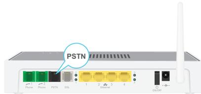
Here you will have to put a filters/splitter between the telephone outlet and your Thomson Gateway.
