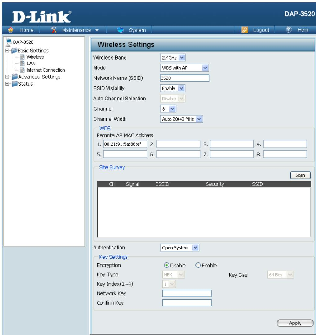
In WDS with AP mode, the DAP-3520 wirelessly connects multiple networks while still functioning as a wireless AP.
