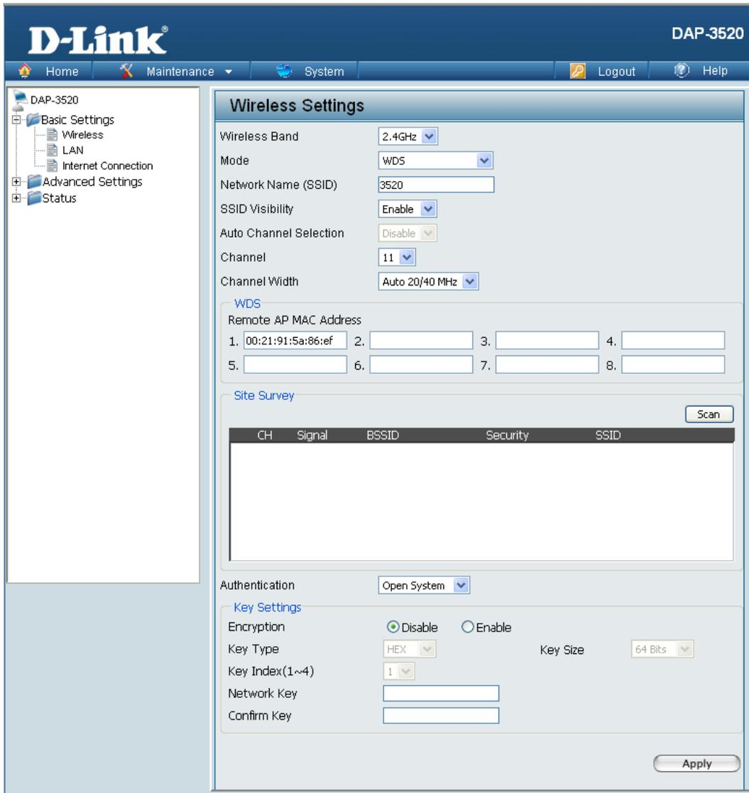
In WDS mode, the DAP-3520 wirelessly connects multiple networks, without functioning as a wireless AP.
