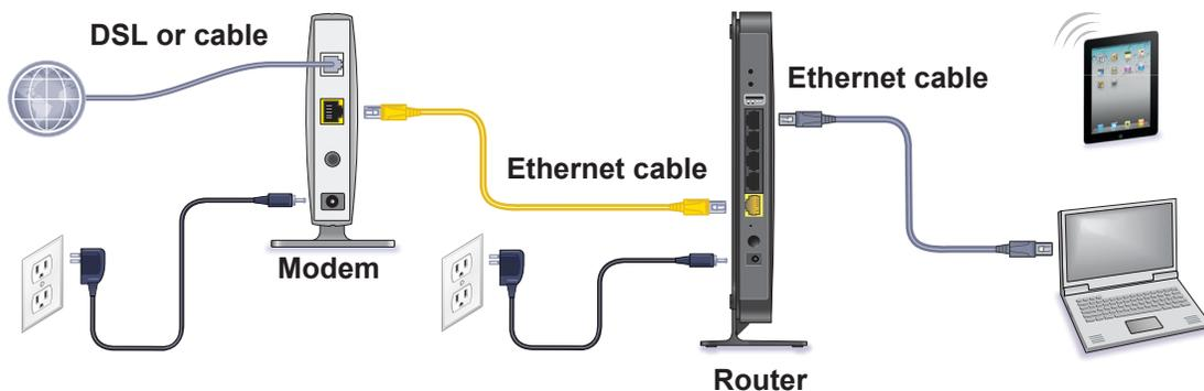
Figure 3. Router cabling
