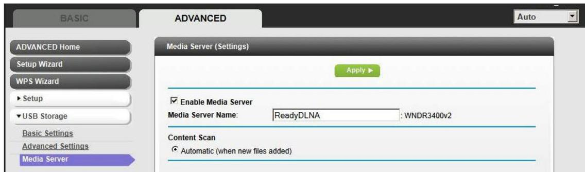
By default, the Enable Media Server check box and the Automatic (when new files are added) radio button are selected. When these options are selected, the router scans for media files whenever new files are added to the ReadySHARE USB hard drive.
