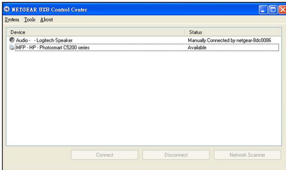
This is the main screen, which shows a device icon, the description for this USB device, and its status.
