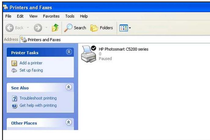
This USB printer is ready. The utility does not need to hold the connection of this USB printer. Once there is any print job for this printer, the USB utility connects to this USB printer automatically, and then prints. After the print job is done, the printer status returns to the Paused state.
