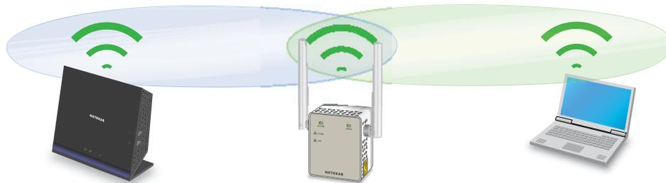
9. Test the extended WiFi range by moving your computer or WiFi device to the area with a poor router WiFi signal:
