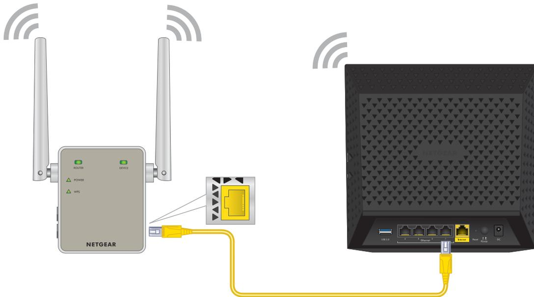
Figure 5. Extender in access point mode
