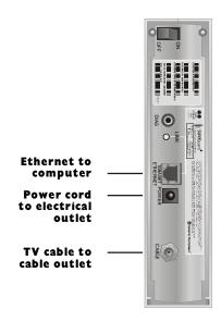
You must call your service provider to activate your service. You need to provide the media access control (MAC) address. This address is found on the barcode label marked HFC MAC ID on the rear panel. The address format is 00:20:40:00:00:00.
