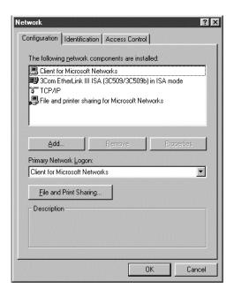
The SB2100 contains all necessary software. You don't need to configure the cable modem but you must configure your computer for TCP/IP and check for an IP address. Your service provider may provide additional instructions for setting up your computer. The following basic instructions are for Windows™ 95 or Windows 98. If you are using a different operating system, refer to that user guide.
