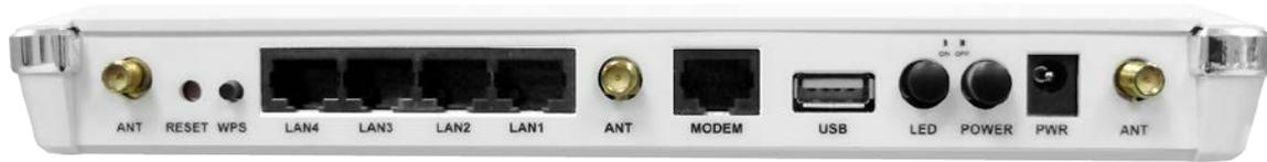
**Antenna Connectors:** RJ-SMA antenna connectors. Attach the included high gain antennas to these connectors.
