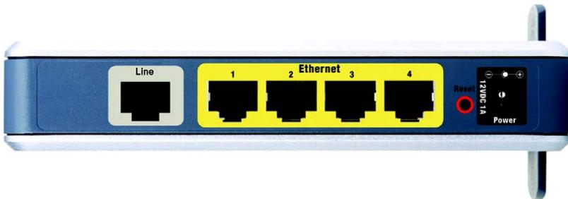
Figure 3-1: Ports and Reset Button on Side Panel
