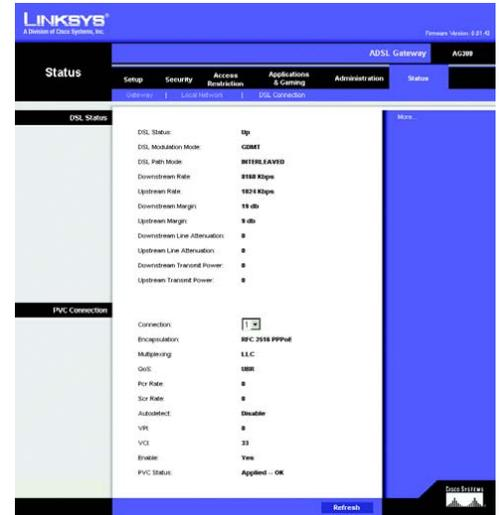
Figure 5-46: DSL Connection
