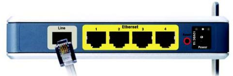
Figure 4-1: Connect the ADSL Line
