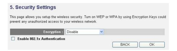
Choose the Encryption type you're using from the drop-down list. There are three types of Encryption:
