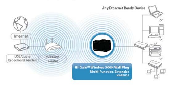
Access Point: The HWREN25 will broadcast a Wireless signal for other computers and devices to connect to. Must be plugged into the router or network after setup.
