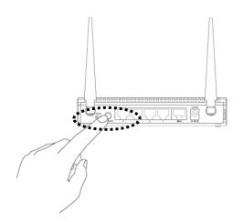
NOTE: this WPS button position on access point is an example. Different devices may have different WPS button position.
