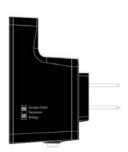
Insert this device into a power outlet in the wall, and switch the Wireless HWREN25's power switch to '**ON**'. You should see '*Power*' LED light up in a few seconds. If not, please check if the power outlet you're using is working.
