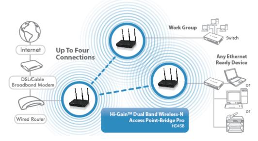
**AP Bridge WDS**: Wireless Distributing System. This allows you to create a wireless network using up to four HD45B's using the same SSID (wireless name). It will broadcast a WiFI signal.
