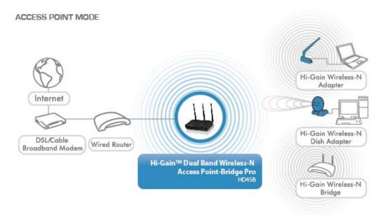
**Station – Infrastructure (Bridge):** The HD45B will allow you connect wired devices wirelessly to an existing wireless router or access point. It will "bridge" these
