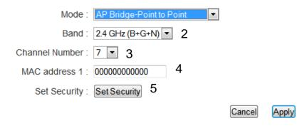
NOTE: Two HD45B's must use the same mode, band, channel number, and security setting!
