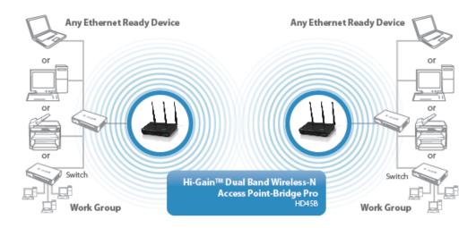
**AP Bridge – Point to Multi-Point:** Similar to AP Bridge – Point to Point, this allows you to connect several HD45B's to one point. No WiFi signal will be broadcast and it will only make a wireless connection between the HD45Bs.
