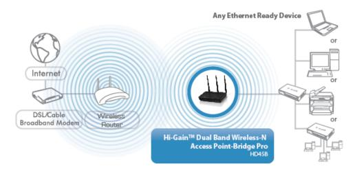
**AP Bridge** – **Point to Point:** Similar to station-infrastructure, this requires two HD45B's on each end. This will create a wireless bridge between these two points. No WiFi signal will be broadcast and it will only make a wireless connection between those two points.
