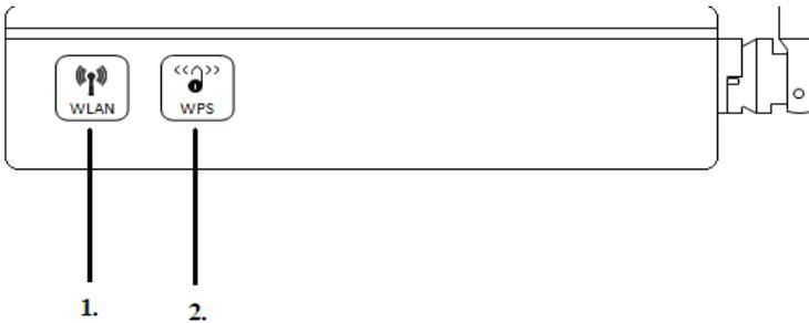
1. **WLAN:** WLAN button: Used to disable the broadcast of the wireless signal.
