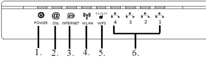
1. **POWER:** Will be lit when the power supply is connected.
