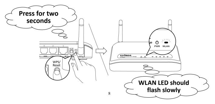
3. The WPS function of the wireless bridge will now be **active for 2 minutes**. So, **within 2 minutes**, please press the WPS button on the wireless router/access point of your root network, to activate its WPS function also.
