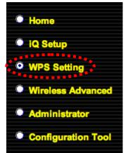
Wi-Fi Protected Setup (WPS) is the simplest way to build a connection between your wireless router/access point and the wireless bridge. You don't have to select an encryption mode and enter a long encryption passphrase – simply press a button on the wireless router/access point and on the wireless bridge, and WPS will do the rest for you.
