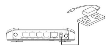
2. Press and hold the WPS button on the wireless bridge for **2 seconds** to activate the WPS function. The WLAN LED should **flash slowly** (two seconds on, two seconds off) to indicate that WPS is in progress.
