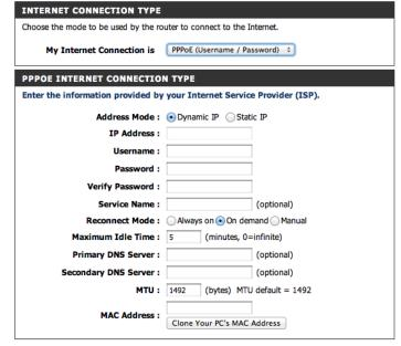
**Maximum Idle** Enter a maximum idle time during which the Internet connection is maintained during inactivity. To disable this feature, enable **Time:** Auto-reconnect.
