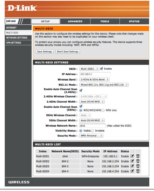
**Enable Auto** This setting can be selected to allow the DIR-640L **Channel Scan** to choose the channel with the least amount of (**5GHz**): interference for the 5GHz band.
