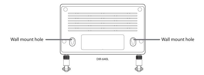
Step 4. Hang the router on the wall by sliding the tops of the screws through the holes on the bottom of the router and then slide to lock into position. Confirm the the router is firmly in place.
