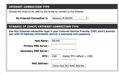
MAC Address: The default MAC Address is set to the Internet port's physical interface MAC address on the Broadband Router. It is not recommended that you change the default MAC address unless required by your ISP. You can use the Copy Your PC's MAC Address button to replace the Internet port's MAC address with the MAC address of your Ethernet card.
