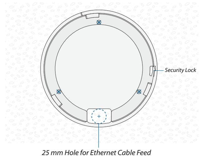
3. Use a 3 mm drill bit to drill the screw holes, and cut or drill the 25 mm hole for the Ethernet cable feed.
