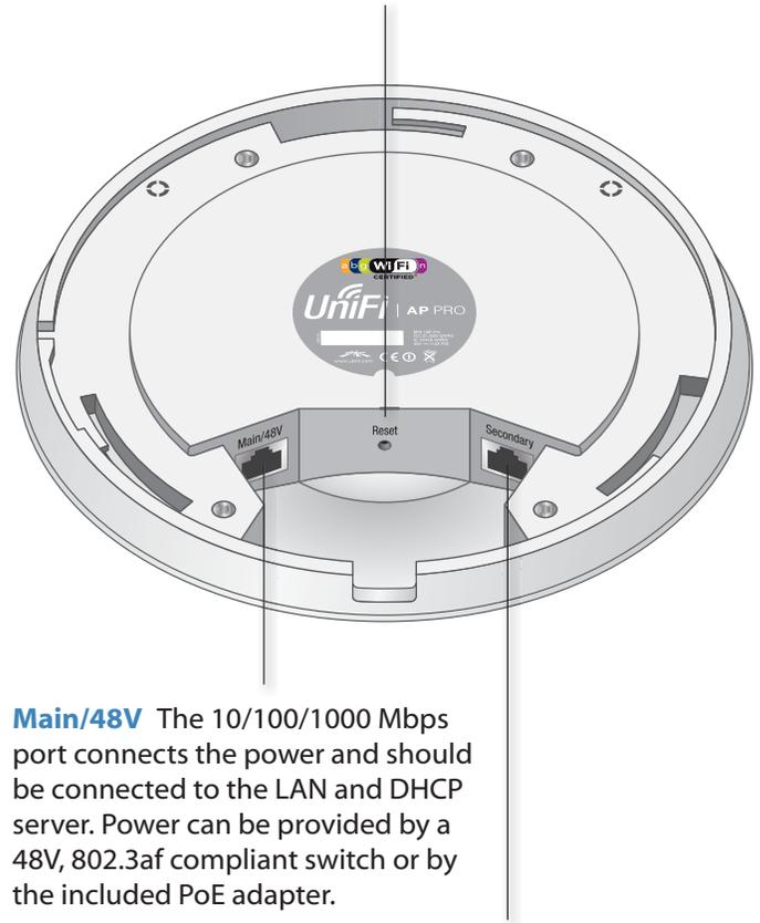
**Main/48V** The 10/100/1000 Mbps port connects the power and should be connected to the LAN and DHCP server. Power can be provided by a 48V, 802.3af compliant switch or by the included PoE adapter.
