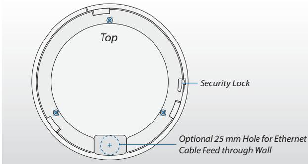
3. (Optional) If your Ethernet cable feeds through the wall, cut or drill a circle that is approximately 25 mm in size and lines up with the cable feed slot.
