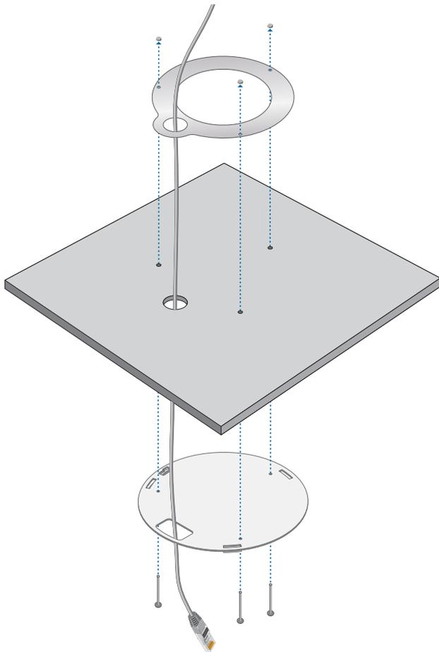
5. Feed the Ethernet cable through the 25 mm hole.
