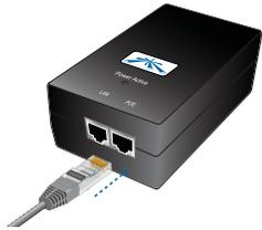
2. Connect an Ethernet cable from your LAN to the Ethernet port labeled **LAN** on the *PoE GigE Adapter*.
