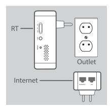
2. Connect one end of your existing Ethernet cable into the Ethernet port of your cable/DSL modem or router and then plug the other end of the cable into the Internet port of the GO-RTW-N300. Verify that the Internet LED is lit before continuing.
