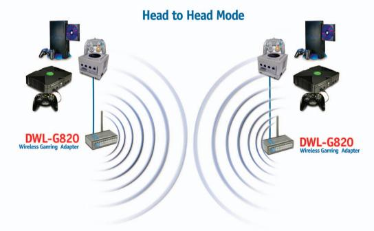
This example illustrates an **Ad-Hoc** setup. Simply connect the DWL-G820 (*refer to the Quick Installation Guide*) to your Ethernet-capable network device (*in this case, a gaming console*) and you will be able to connect wirelessly with other gaming consoles also connected to DWL-G820s.
