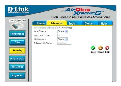
The D-Link DWL-2100AP allows you to balance the distribution of wireless client connections across multiple access points. Using load balancing, you can prevent scenarios where a single access point in your network shows performance degradation because it is handling a disproportionate share of the wireless traffic.
