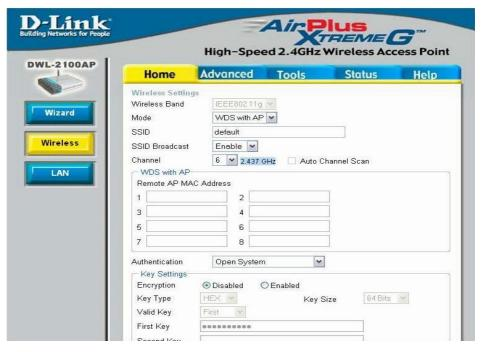
WDS (Wireless Distribution System) with AP mode can set APs to work as PtP/PtMP Bridge and Access Point function simultaneously with the same security setting. But all APs need to set as the same SSID.
