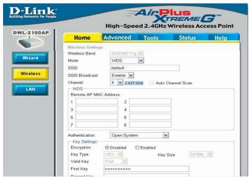
WDS (Wireless Distribution System) mode can set APs to work as PtP/PtMP Bridge. But all APs need to set as the same SSID.
