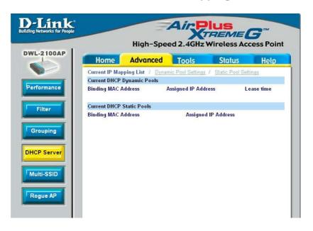
This screen displays information about the current DHCP dynamic and static IP address pools. This information is available when you enable the DHCP function of the DWL-2100AP and assign dynamic and static IP address pools.
