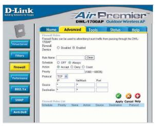
Firewall Rules is an advanced feature that is used to deny, allow or count traffic that passes through the DWL-1700AP. The Firewall Rules that you create will appear in the list at the bottom of the page. Please be sure to Click Apply, after you have made changes or additions.
