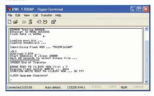
Key-in **reboot** and press **Enter** to let the new boot code activate. After rebooting and when showing **EDORAM Testing**, press **X** to enter console mode again.
