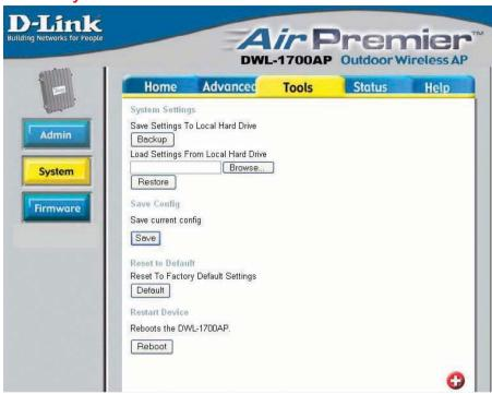
The current system settings can be saved as a file onto the local hard drive. The saved file or any other saved setting file can be loaded back on the DWL-1700AP. To reload a system settings file, click on **Browse** to browse the local hard drive and locate the system file to be used. You may also reset the *Wireless Access Point* back to factory settings by clicking on **Default.**
