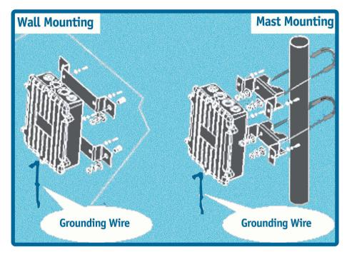
The DWL-1700AP can be mounted on the side of a building or mounted to a mast as shown above. A wall mount is a convenient location if the roof overhang is not excessive and/or the location is high enough to provide a clear line of sight.
