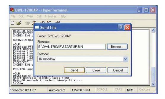
When **XMODEM End of Transfer** and **Erase Root FW (X.BIN) NOW (Y/y):** appears, type **Y** to update Flash.
