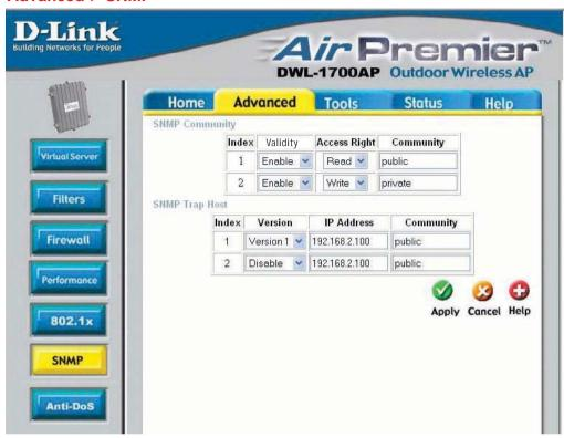
SNMP (Simple Network Management Protocol) is a widely used network monitoring and control protocol that reports activity on each network device to the administrator of the network. SNMP can be used to monitor traffic and statistics of the DWL-1700AP.
