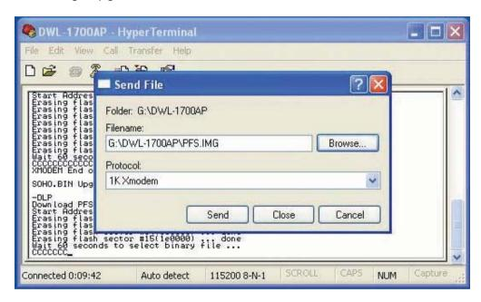
Key in **DLB** and press **Enter** to upgrade the BIOS. When **CCC...** appears, select **Transfer** > **Send File.**
