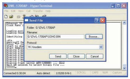
Key-in **DLP** and press **Enter** to erase the old Web image and when **CCC...** appears, select **Transfer** > **Send File**.
