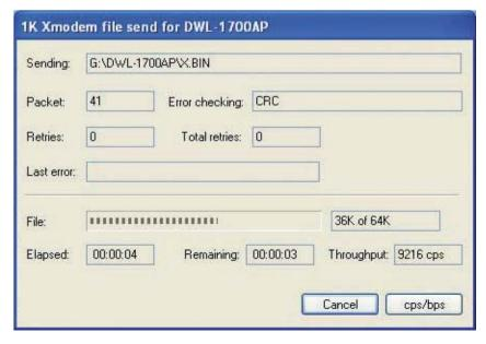
When XMODEM End of Transfer & ERASE ROOT FW (X.BIN) NOW (Y/y): appears, type Y to update Flash.
