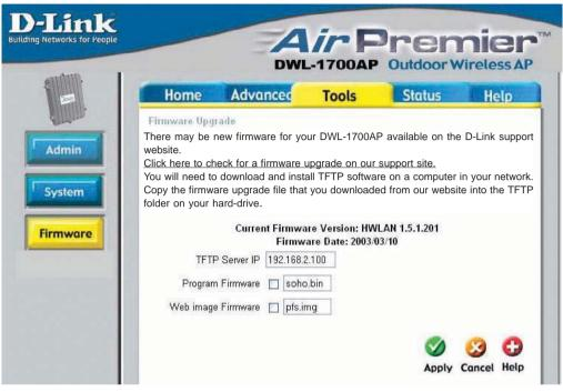
You can upgrade the firmware of the Access Point here. Make sure the firmware you want to use has been copied into the TFTP folder on the computer in your network which has the TFTP software installed. Remember the names of the firmware upgrade files. Please check the D-Link support site for firmware updates at http://support.dlink.com. You can download firmware upgrades to your hard drive from the D-Link support site.
