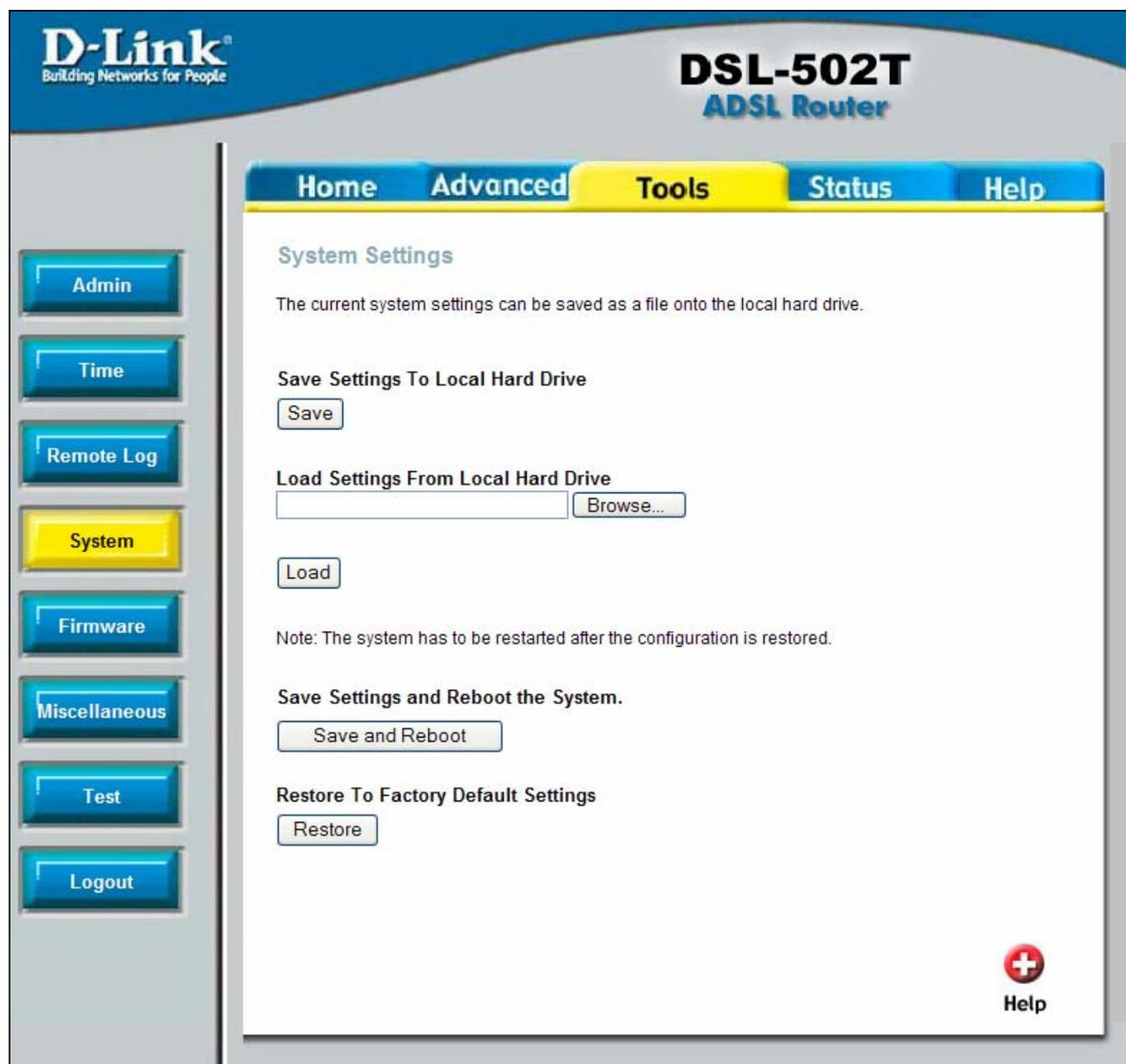
The screenshot shows the web interface for the DSL-502T ADSL Router. The top navigation bar includes tabs for Home, Advanced, Tools (highlighted in yellow), Status, and Help. On the left side, there is a vertical menu with buttons for Admin, Time, Remote Log, System (highlighted in yellow), Firmware, Miscellaneous, Test, and Logout. The main content area is titled "System Settings" and contains the following sections:
