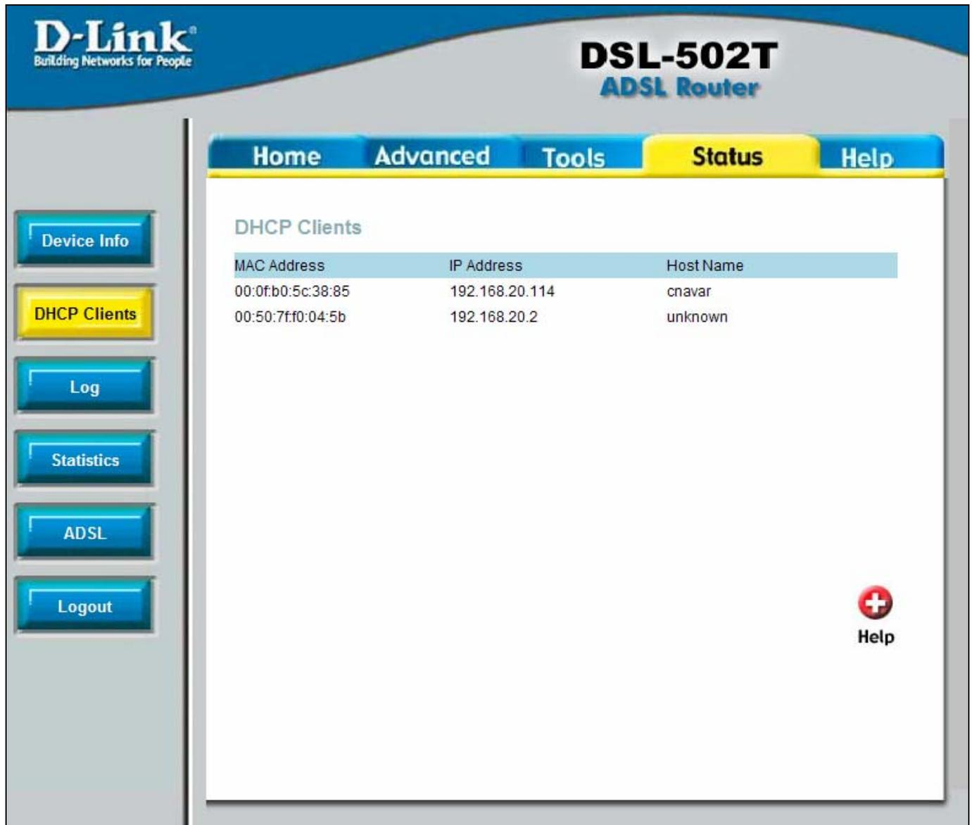
The screenshot shows the web interface of a D-Link DSL-502T ADSL Router. The top navigation bar includes 'Home', 'Advanced', 'Tools', 'Status' (highlighted), and 'Help'. The left sidebar contains buttons for 'Device Info', 'DHCP Clients' (highlighted), 'Log', 'Statistics', 'ADSL', and 'Logout'. The main content area displays the 'DHCP Clients' table with the following data:
