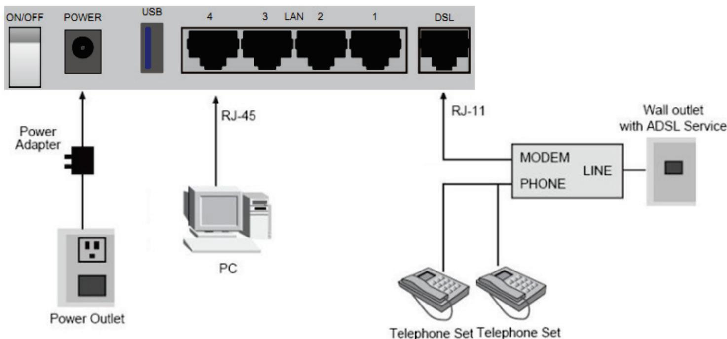
**Step 1** Connect the **DSL** port of the router and the Modem port of the splitter through a telephone cable; connect the phone to the phone port of the splitter through a telephone cable; and connect the Line port of the splitter to the uplink telephone jack on the wall.
