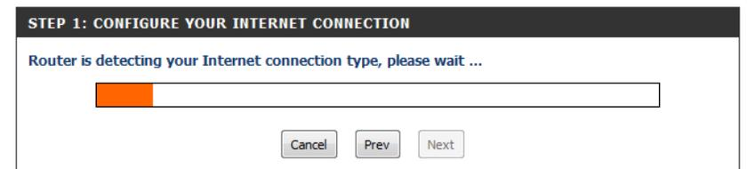
If the router does not detect a valid Ethernet connection from the Internet port, this screen will appear. Connect your broadband modem to the Internet port and then click **Connect**.
