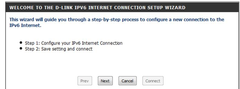
The router will attempt to detect whether its possible to obtain the IPv6 Internet connection type automatically. If this effort is successful, the user will be guided through the input necessary for the connection type found.
