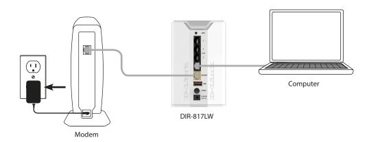
5. Plug the power adapter into your router and connect to an available power outlet or surge protector. If the Power LED does not light up, press the Power button on the back of the router.
