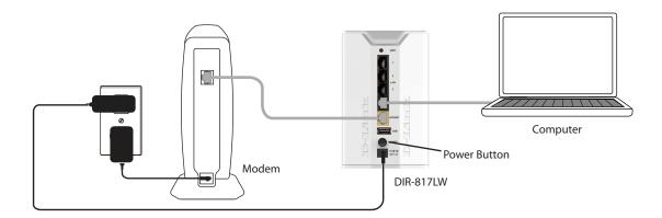
6. After the router has powered up, verify that the power (green) and Internet (orange or green) LEDs are both lit. Skip to "Configuration" on page 13 to learn about your configuration options. If you initially choose not to connect to the Internet, later you can use the "Internet Connection Setup Wizard" on page 32.
