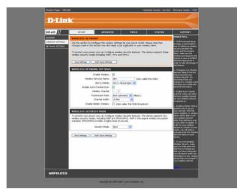
Enable Auto The Auto Channel Scan setting can be selected to allow the DIR-605 to choose the channel with the least amount of interference.
