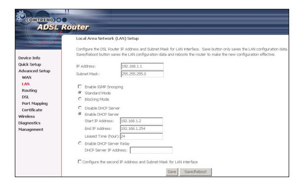
**Enable IGMP Snooping:** Enable /Disable the function that is IGMP Snooping.
