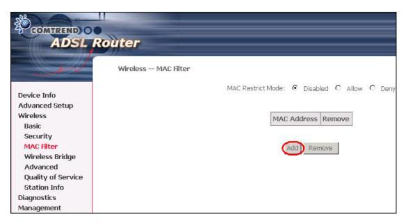
After choosing the Add button, the following screen appears. Enter the MAC address and click **Apply** to add the MAC address to the wireless MAC address filters.
