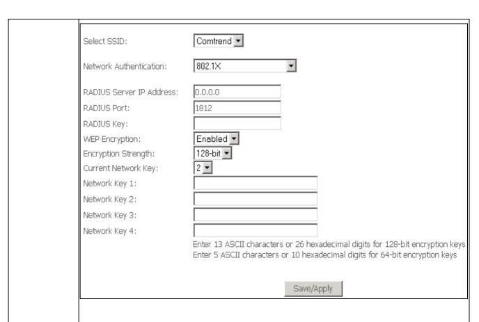
Select the Current Network Key and enter 13 ASCII characters or 26 hexadecimal digits for 128-bit encryption keys and enter 5 ASCII characters or 10 hexadecimal digits for 64-bit encryption keys.
