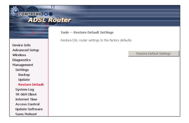
**NOTE 1:** This entry has the same effect as the hardware reset-to-default button. The CT-5361T board hardware and the boot loader support the **reset to default** button. If the reset button is continuously pushed for more than 5 seconds, the boot loader will erase the entire configuration data saved on the flash memory.
