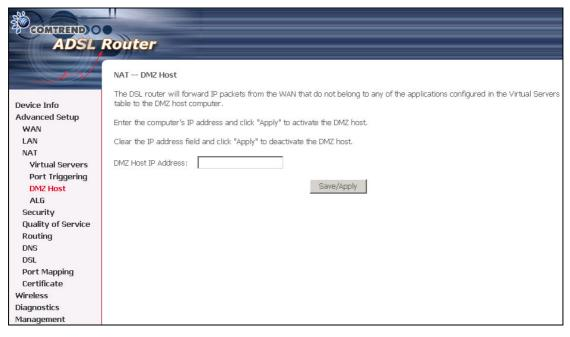
Enter the computer's IP address and click "Apply" to activate the DMZ host. Clear the IP address field and click "Apply" to deactivate the DMZ host.
