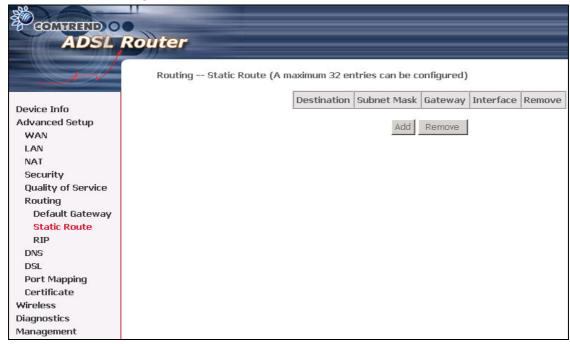
To add static route, click the **Add** button to display the following screen. Enter the destination network address, subnet mask, gateway AND/OR available WAN interface then click **Save/Apply** to add the entry to the routing table.
