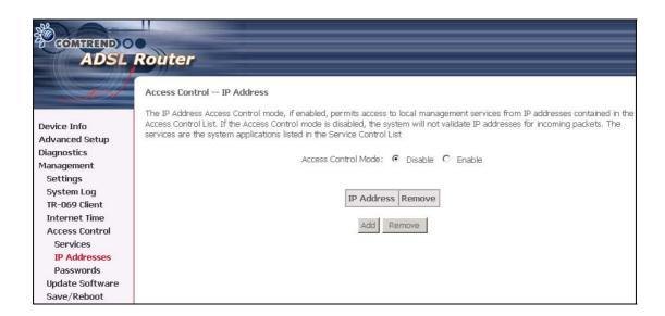
Before you enable it, configure the IP addresses by clicking the **Add** button. Enter the IP address and click **Save/Apply** to allow the PC with this IP address managing the DSL Router.
