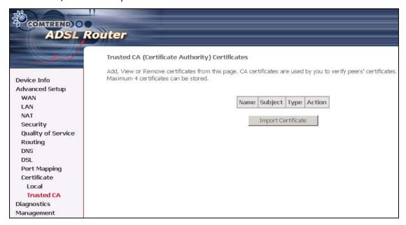
Click **Import Certificate** to paste the certificate content of your trusted CA. Generally speaking, the certificate content will be provided by your vendor/ISP/ITSP and is used to authenticate the Auto-Configuration Server (ACS) that the CPE will connect to.
