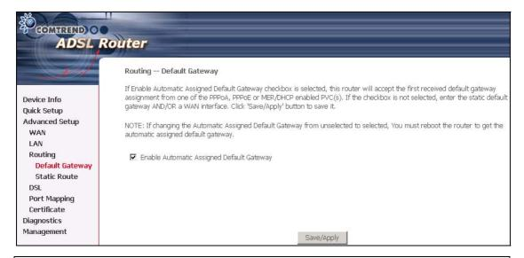
**NOTE:** If changing the Automatic Assigned Default Gateway from unselected to selected, You must reboot the router to get the automatic assigned default gateway.
