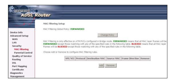
Choose **Add** or **Remove** to configure MAC filtering rules. The following screen pops up when you click **Add**. Create a filter to identify the MAC layer frames by specifying at least one condition below. If multiple conditions are specified, all of them take effect. Click **Apply** to save and activate the filter.
