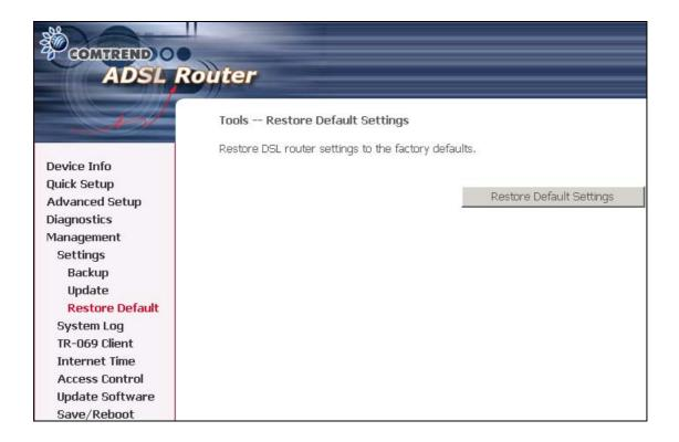
**NOTE:** This entry has the same effect as the hardware reset-to-default button. The CT-5071T board hardware and the boot loader support the **reset to default** button. If the reset button is continuously pushed for more than 5 seconds, the boot loader will erase the entire configuration data saved on the flash memory.
