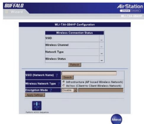
Once you've configured these basic settings (especially *SSID*, the *Encryption Mode*, and the *Encryption Key*), the Ethernet Converter should be able to connect to your other wireless devices. To continue configuring advanced settings, please skip to the next page.
