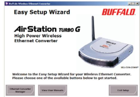
The Ethernet Converter Manager software will run. If the search doesn't begin automatically, select the *Search for an Ethernet Converter* option from the *Edit* drop down menu.
