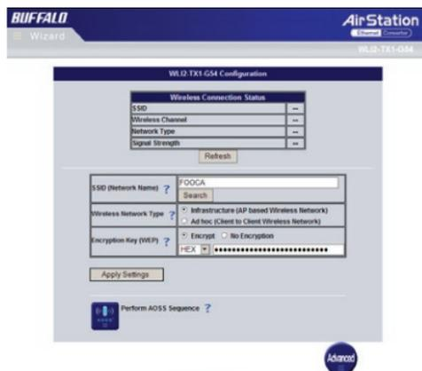
If the wireless network you are attempting to connect to is not broadcasting its SSID, then you will be required to manually enter the SSID into the SSID field. After the field is populated with the proper SSID, press the *Apply Settings* button.
