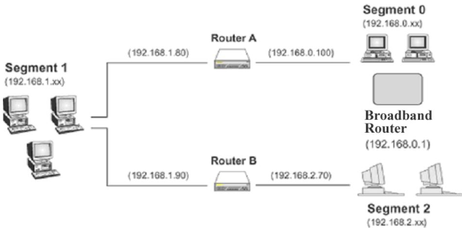
Figure 47: Routing Example
