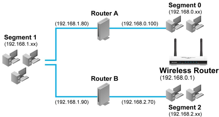
**Figure 64: Routing Example**
