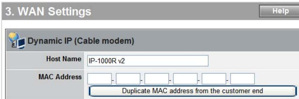
The screenshot shows the '3. WAN Settings' window with a 'Help' button. The selected option is 'Dynamic IP (Cable modem)'. The 'Host Name' field contains 'IP-1000R v2'. The 'MAC Address' field consists of six empty boxes separated by dashes. Below the MAC Address field is a button labeled 'Duplicate MAC address from the customer end'.
