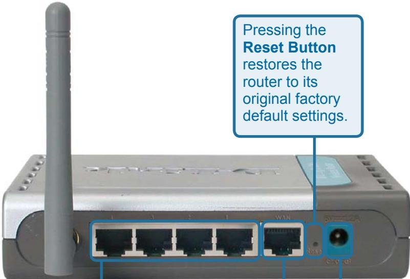
Pressing the **Reset Button** restores the router to its original factory default settings.
