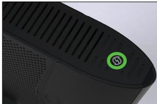
The Extender is now synced with the gateway/modem's Wi-Fi settings. Unplug the Extender and its power cable and continue on to the next section of this chapter, "Connecting the Extender."
