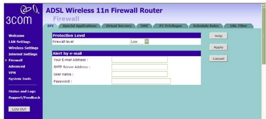
Figure 69 Low and Medium Level Firewall Protection Screen
