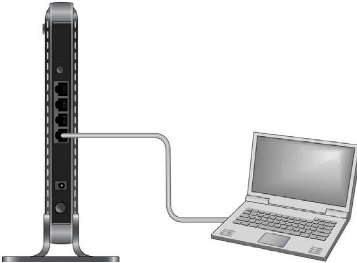
Figure 4. Using an Ethernet cable to connect the extender to a PC
