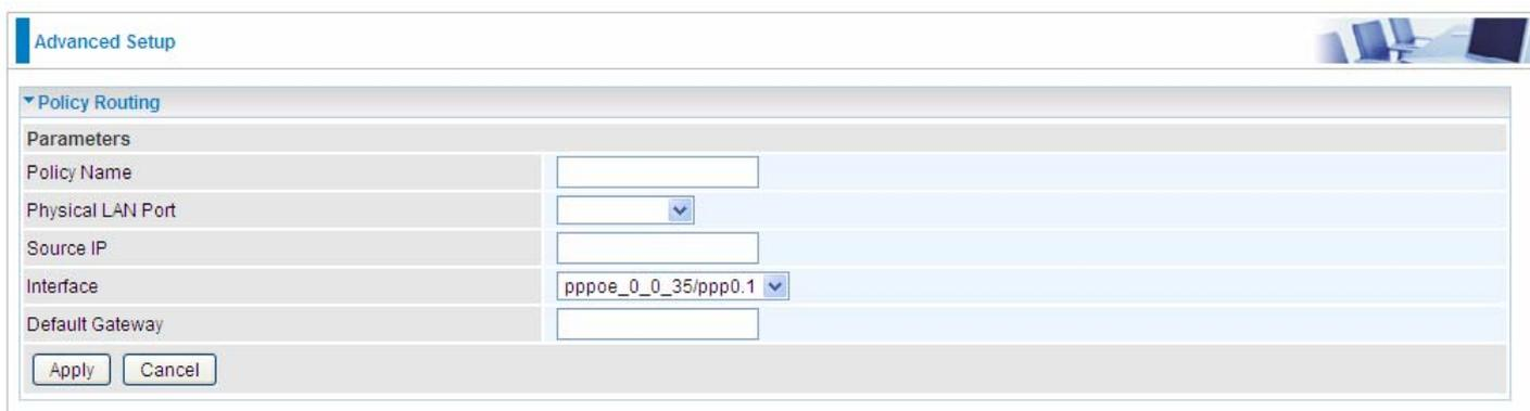
The screenshot shows the 'Advanced Setup' interface with the 'Policy Routing' section expanded. The configuration form contains the following fields: Policy Name (text input), Physical LAN Port (dropdown menu), Source IP (text input), Interface (dropdown menu with 'pppoe\_0\_0\_35/ppp0.1' selected), and Default Gateway (text input). At the bottom are 'Apply' and 'Cancel' buttons.
