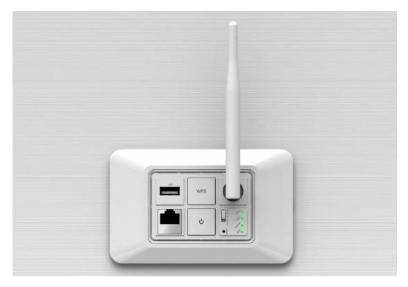
When this product is used as an access point, the IP address has to be changed. The default IP under AP mode is 192.168.1.254.
