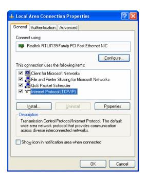
**Step 4-1.** For getting IP automatically if you are one of the users under WA982N Broadband Router, please skip **Use the following IP address** and then select **Obtain an IP address automatically** and **Obtain DNS server address automatically** and then click on **OK** button.
