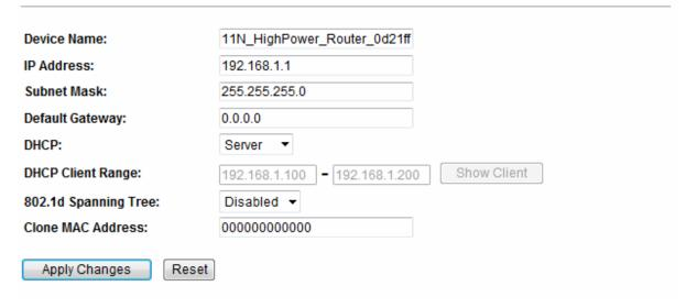
**Step 6.** Doing the same way to setup the MAC address in the paired device. Launch the UT to the menu "**WDS settings**" of the paired device, and input router's MAC address. Click **Apply Changes** to save the setting data.
