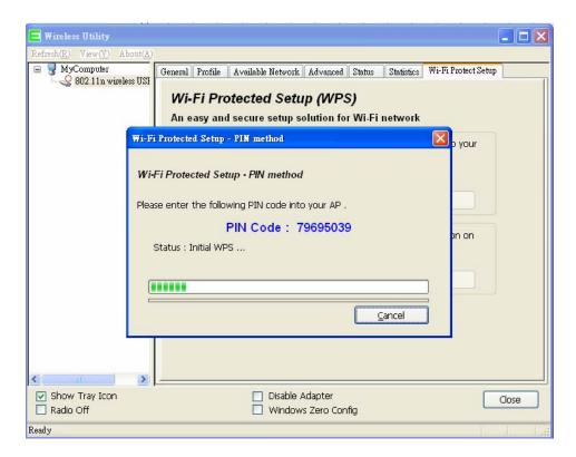
(2.) Open menu "Wi-Fi Protected Setup" of WA982N Broadband Router, input the PIN number from the wireless card then click **Start PIN**.
