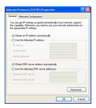
**Step 4-2.** For getting IP manually in order to specify a Virtual Server, such as Print Server, FTP Server and so on, please skip **Obtain an IP address automatically** and then select **Use the following IP address**. And the following default setting of WA982N Broadband Router should be noted:
