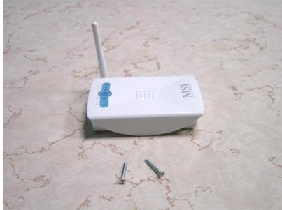
**Step 2** Hammer the screws into the ceiling or the wall.
