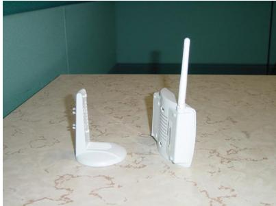
**Step 2** Locate the mounting holes on the rear panel of the AP11B and align them to the hooks of the stand.
