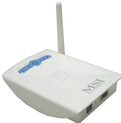
MSI AP11B wireless access point is IEEE802.11b compliant, and connects one or more wireless enabled computers to an Ethernet network or Cable/xDSL modem for high speed connection, anywhere in your home or office.
