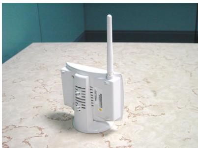
**Step 4** Hold and slide the AP11B to either right or left to secure the access point in place.
