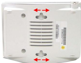
**Step 5** The wall- or ceiling-mounted installation is completed. To have the maximum wireless coverage, point the antenna vertically downward for ceiling-mounted installation. For wall-mounted installation, point the antenna vertically upward.
