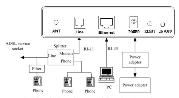
Fig 2-2 Connection Diagram (Connecting a telephone set before the splitter)
