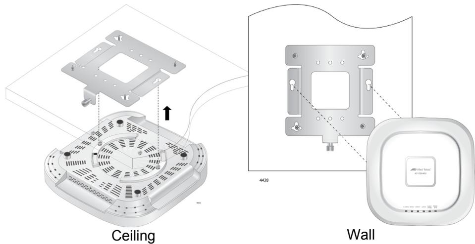
Figure 16. Align/Insert Access Point into Mounting Bracket
