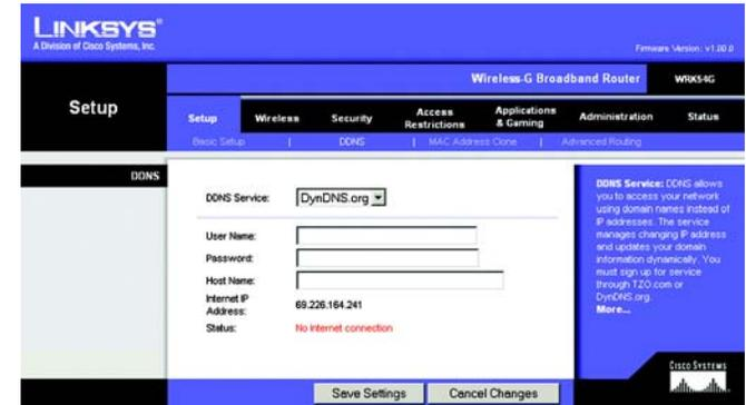
Figure 5-13: Setup Tab - DDNS - DynDNS account
