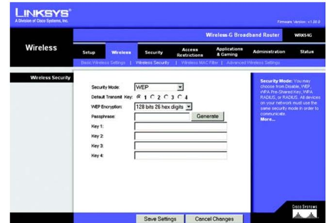
**Figure 5-24: Wireless Tab - Wireless Security (WEP)**
