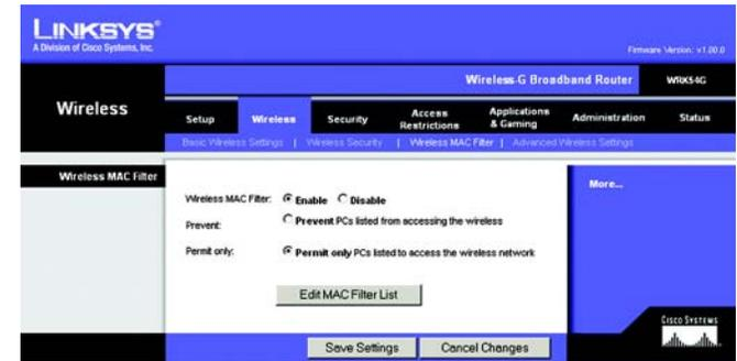
Figure 5-25: Wireless Tab - Wireless MAC Filter
