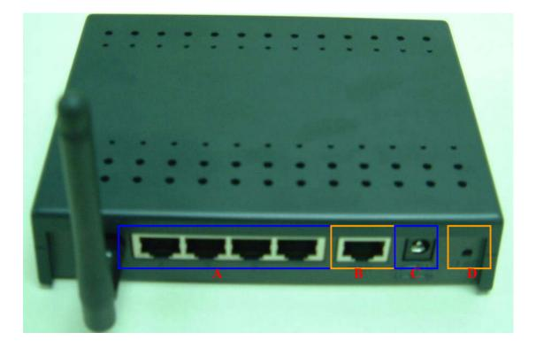
**A** (LAN Ports): automatically sense the cable type when connecting to Ethernet-enabled computers.
