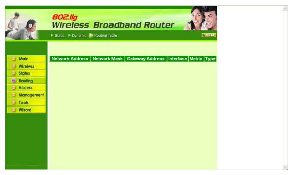
Network Address: Displays the network IP address of the connected node. Network Mask: Displays the network (subnet) mask of the connected node. Gateway Address: Displays the gateway address of the connected node. Interface: Displays whether the node is connected via a WAN or LAN. Metric: Displays the metric of the connected node. Type: Displays whether the node has a static or dynamic IP address
