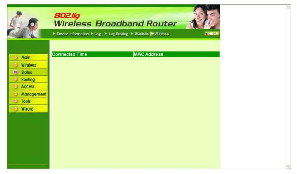
**Connected Time:** Displays how long the wireless device has been connected to the LAN via the router.
