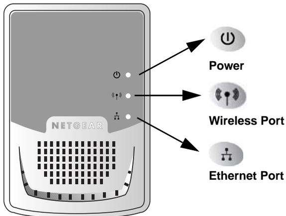
**Figure 2-2: WGR101 Front Panel**
