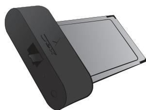
Slide your **Aris Wireless card** into the slot and press firmly to seat it securely. If you feel any resistance, the card is probably backwards. Just turn it around and try again.
