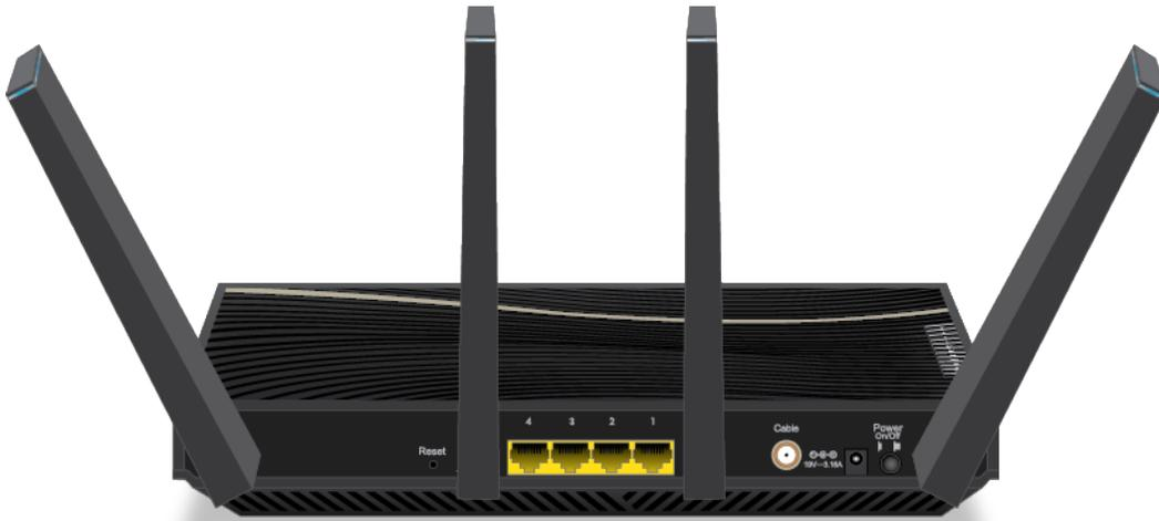
**Figure 2. Modem router rear panel**
