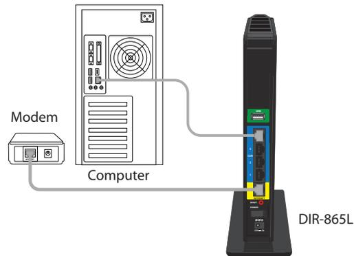
5. Reconnect the power adapter to your cable or DSL broadband modem and wait for two minutes.
