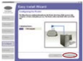
5.1 The Wizard will now transfer all of the configuration information to the Router. This will take approximately one minute. During this time, do not turn off the Router or computer. The Router will restart itself at the end of this step.
