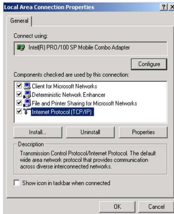
4. Configure the IP address for the Ethernet connection in the Internet Protocol (TCP/IP) Properties dialog box.
