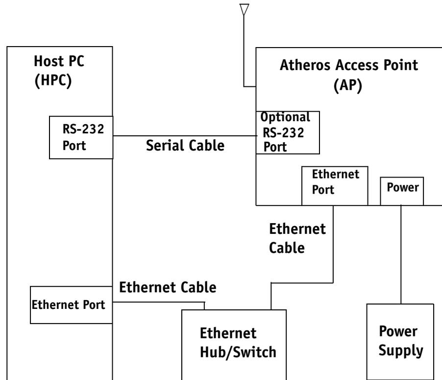
Figure 2-1. Access Point to HPC Connections
