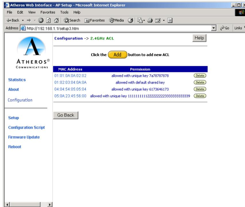
Figure A-8. 2.4 GHz Access Control List Configuration Window
