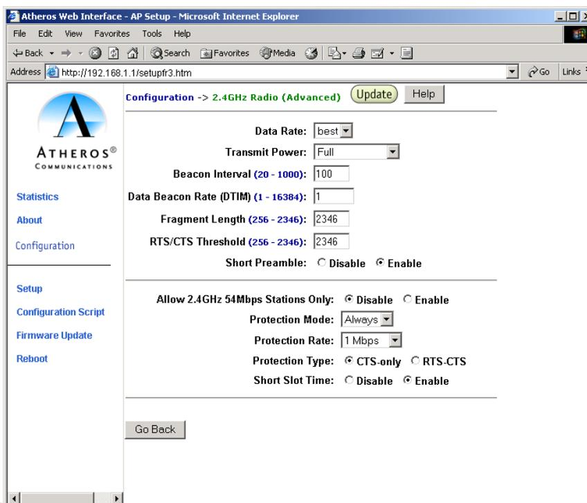
Figure A-11. 2.4 GHz Radio Advanced Configuration Window
