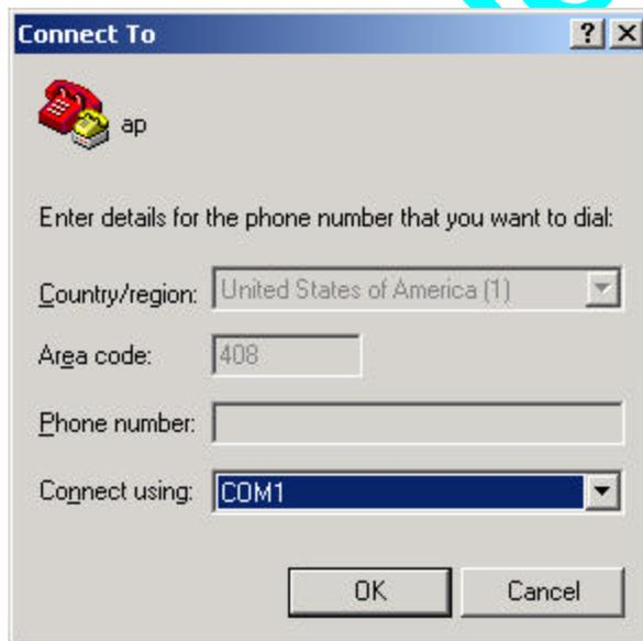
9. Set COM port settings to 9600 Bits per second, 8 Data bits, None Parity, 1 Stop bits, and no Flow control. Click OK, and plug the AP power supply into the power source to start the connection.
