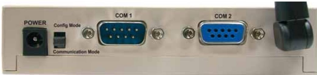
**POWER** Plug in the power adapter of 12V DC/1A into the power port.
