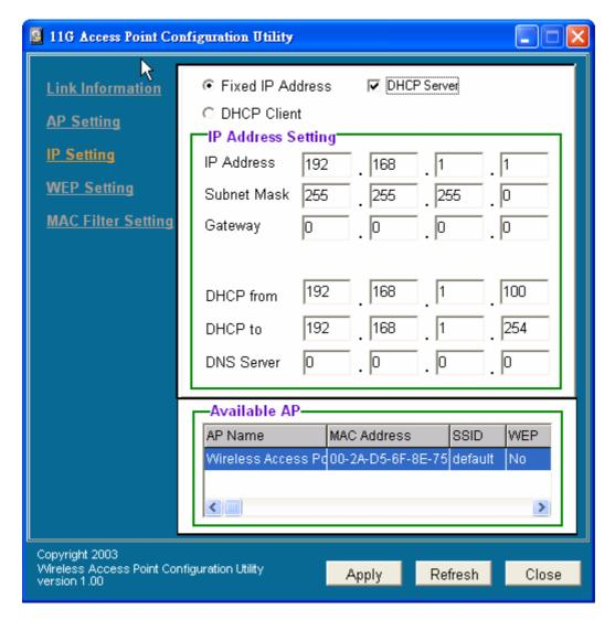
Fixed IP Address: Users can assign a fixed IP address to this AP manually.
